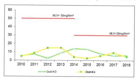
\*MLV=50 mg/Nm³ – Maximum limit value according to national law for emissions \*MLV=30 mg/Nm³ – Maximum limit value accepted from USJE in the A-IPPC
